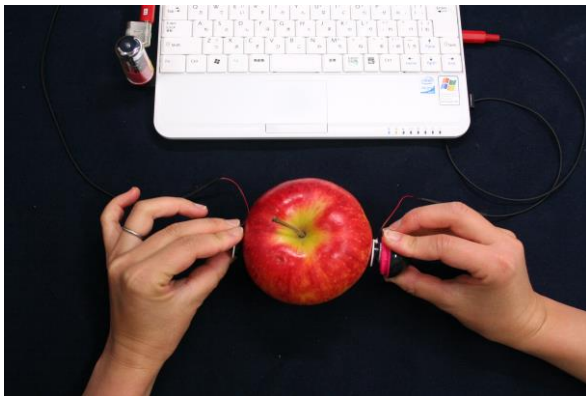
Fig. 3 Measurement of resonant frequency of the tested material. Right, vibration part; left, receiver.
