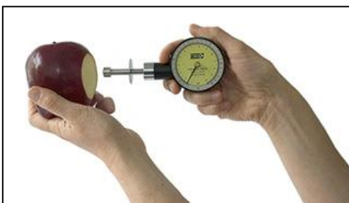
Fig. 1 Puncture test with a fruit pressure tester. to the market.
